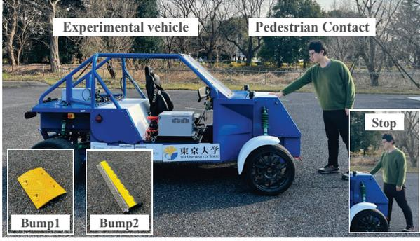
Fig. 2: Experimental vehicle FPEV-5. The Bump1 is round with the width of 50 cm, the depth of 35 cm, and the height of 4.5 cm. The Bump2 is trapezoidal inshape with the topbase of 18 cm, the bottom of 30 cm, and the height of 5.3 cm .
