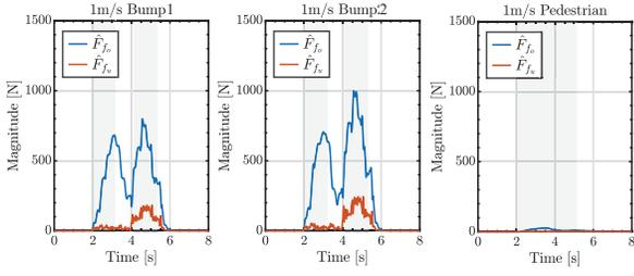
Fig. 7: Simulation results of  $\hat{F}_{f_o}$  and  $\hat{F}_{f_u}$  when contacting and passing over a bump or pedestrian at a constant speed.
