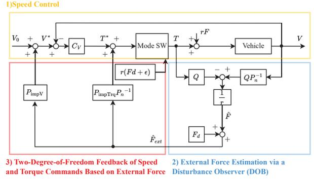
Fig. 3: Block diagram of the conventional method.
