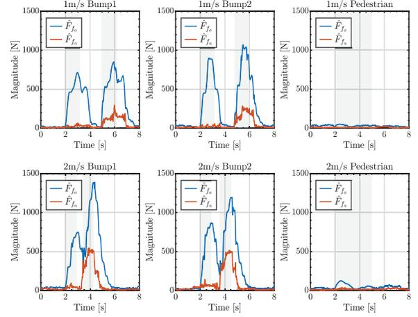
Fig. 8: Experimental results of  $\hat{F}_{f_o}$  and  $\hat{F}_{f_u}$  when contacting and passing over a bump or pedestrian at a constant speed.
