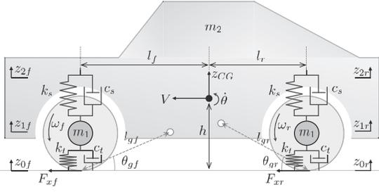
Fig. 4: Vehicle motion model.
