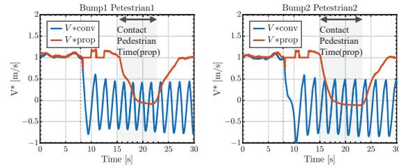
Fig. 11: Experimental results of the velocity command  $V^*$  of EV.
