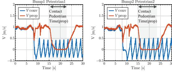
Fig. 10: Experimental results of the wheel velocity  $V$  of EV.
