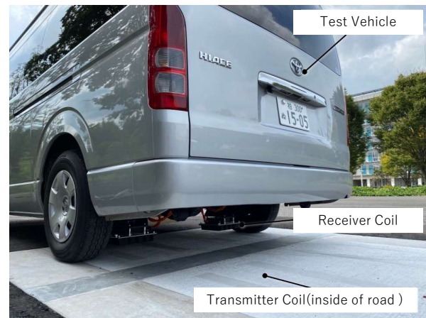
Fig. 2. Demonstration vehicle for DWPT utilized in Kashiwa, Japan.
