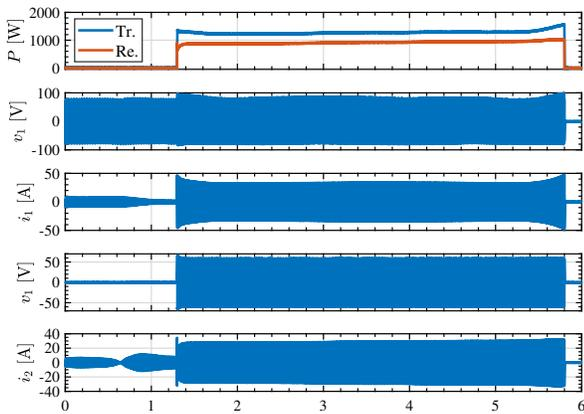
Fig. 11: Experimental results with sensorless detection when gap = 10 cm and pitch = 5 deg.
