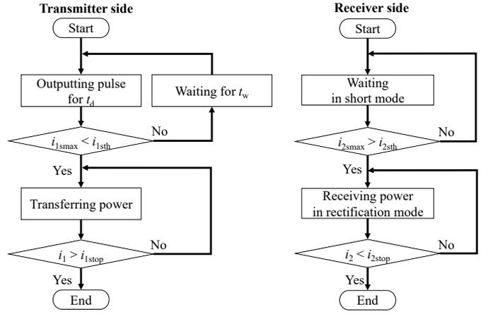
Fig. 3: Flowchart of sensorless receiver coil detection.
