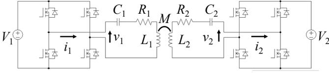
Fig. 2: Series-series type WPT circuit diagram.
