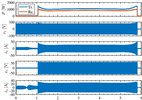
Fig. 7: Experimental results with sensorless detection when gap = 8 cm and pitch = 0 deg.
