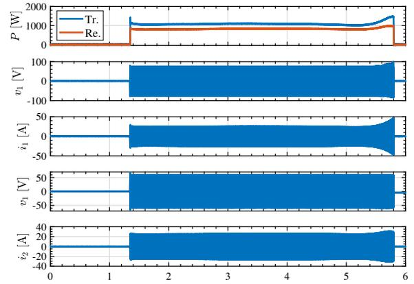
Fig. 8: Experimental results with position-sensor-based detection when gap = 8 cm and pitch = 5 deg.
