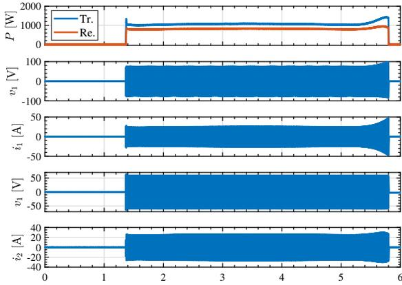
Fig. 6: Experimental results with position-sensor-based detection when gap = 8 cm and pitch = 0 deg.
