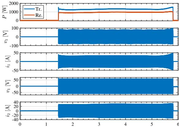
Fig. 10: Experimental results with position-sensor-based detection when gap = 10 cm and pitch = 5 deg.
