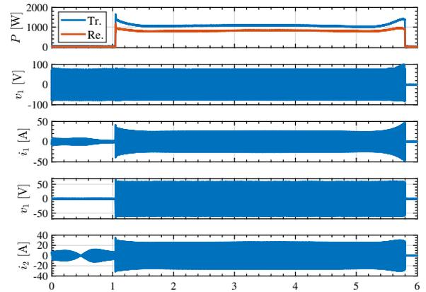
Fig. 9: Experimental results with sensorless detection when gap = 8 cm and pitch = 5 deg.
