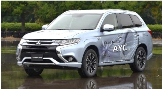
Figure 17. Experimental vehicle equipped with TDA-TVD. TDA-TVD drives rear wheels using two electric motors.
