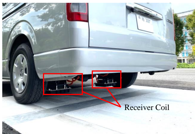
Fig. 2 Test Vehicle with DWPT System
