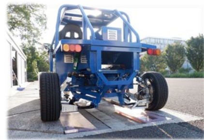
Fig.3 EV and DWPT system for EVs.
