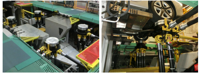
(a) Four-poster test rig. (b) Magnified view.
