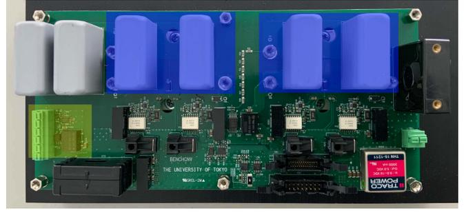
Fig. 5. Photograph of the experimental converter board.
