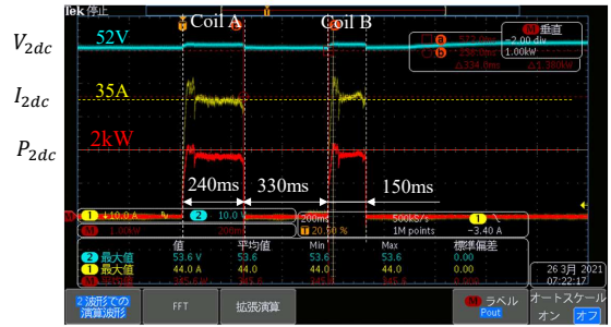
Fig. 17. DWPT Test Result on VLR(10km/h)
