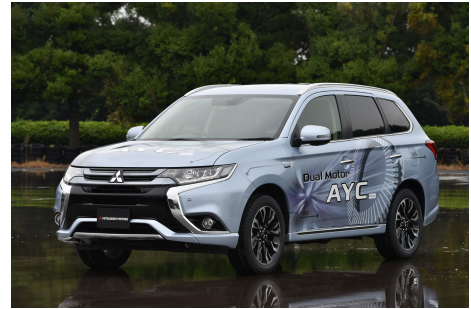
Fig. 7 Experimental vehicle equipped with TDA-TVD. TDA-TVD drives rear wheels using two electric motors.
