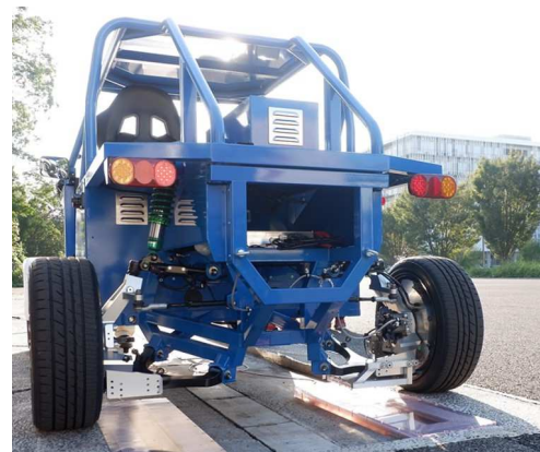
Fig. 1. The experimental vehicle for DWPT
