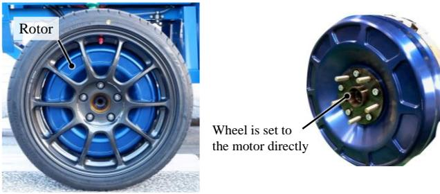
Fig.5 Structure of Motor
