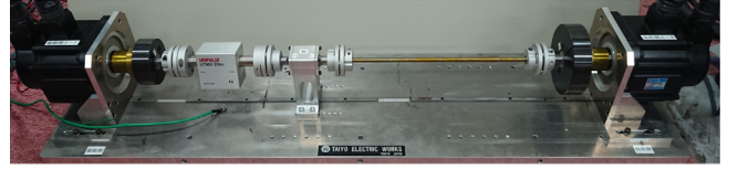
(a) Photograph of two-inertia system motor bench.
