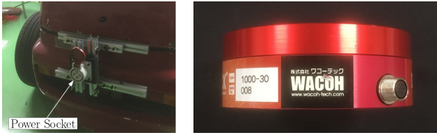
(a) Power socket attached to the experimental vehicle. (b) Force/moment sensor used to measure the actual reaction force/torque.
