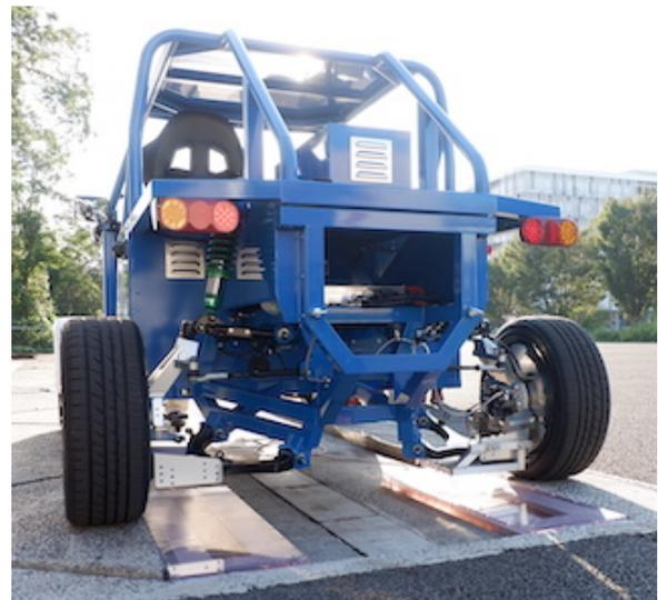
Fig. 1. The third generation wireless in-wheel motor.
