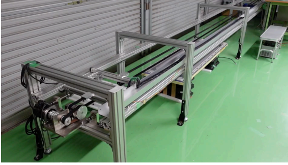
Fig. 8. Experimental setup : In-motion WPT bench. The bench has a moving belt and the receiving coil is put on the bottom of the belt. The transmitting coil is fixed on the ground.
