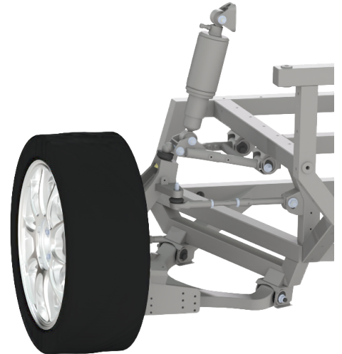
(b) Multibody dynamics model overview.
