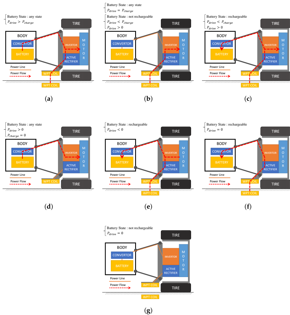
Figure 5. DWPT state of IWM-3. (a) Driving with Energy of Battery and WPT; (b) driving with only energy of WPT; (c) driving and charging with energy of WPT; (d) driving with energy of the battery; (e) charging with energy of regenerating and WPT; (f) charging with energy of WPT; (g) not driving or charging.
