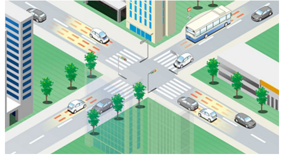
Fig. 1. Semi-dynamic wireless charging system in EVs.
