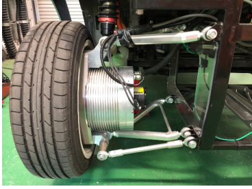
Fig. 3. G-IWM unit with motor-side and load-side encoders.
