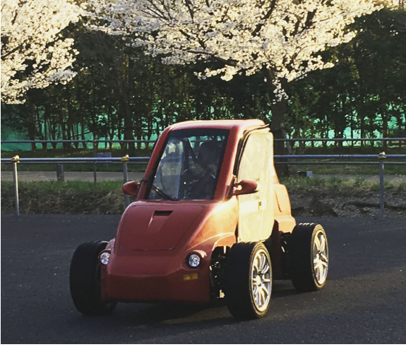
Fig. 1. Vehicle demonstrator FPEV2-Kanon with four individual electric motors.
