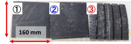
Fig.7 Cut tires used for measurement. (1:inner liner layer , 2:belt layer, 3:tread layer)
