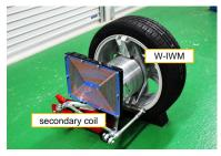
Fig. 10 Secondary side (in-wheel motor side)
