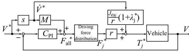
Figure 8: Vehicle speed control system.
