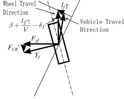
Figure 4: Cornering resistance of front tyre.
