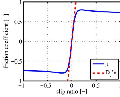
Figure 5:  $\mu$ - $\lambda$  Curve [10].
