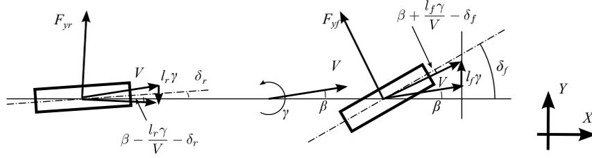
Figure 3: Bicycle model of vehicle dynamics.
