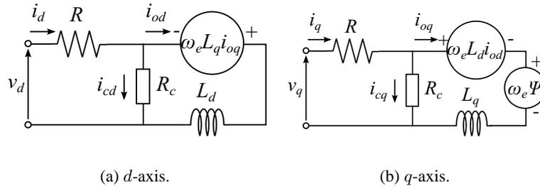
Figure 6: Equivalent circuit of PMSM [12].
