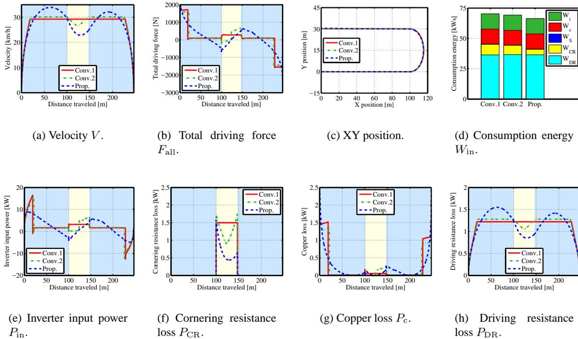
Figure 9: Simulation results (Corner).
