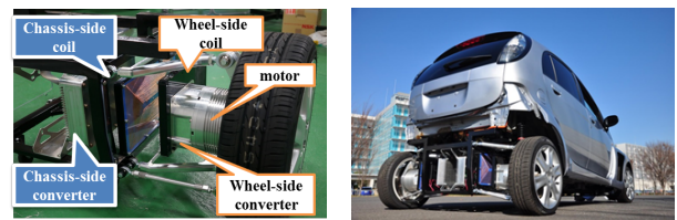
(a) The first trial unit of W-IWM (b) Experimental vehicle
