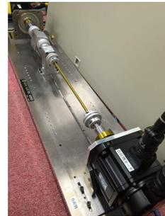
Fig. 1. Outlook of the two-inertia system motor bench.
