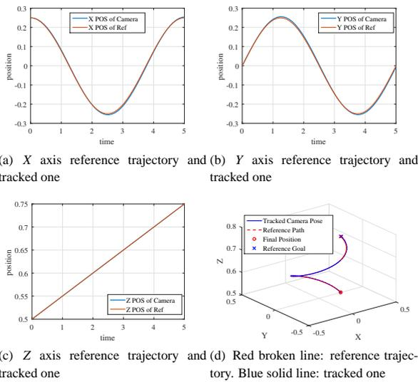
Figure 8: Tracking result using proposed time-invariant jacobian in (7)
