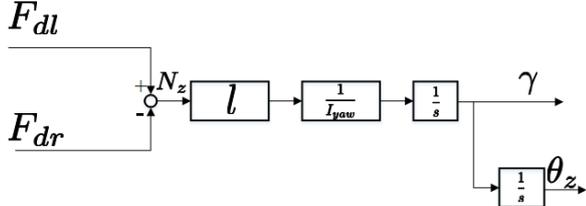
Fig. 6. Block diagram of yaw moment model
