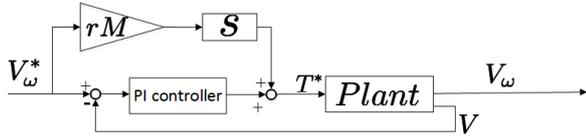
Fig. 7. Block diagram of velocity feedforward controller
