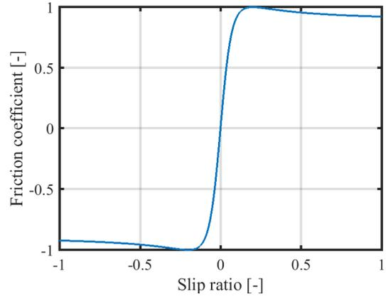
Fig. 4.  $\mu - \lambda$  curve
