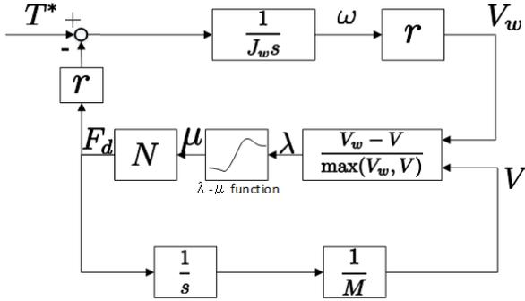
Fig. 5. Block diagram of driving wheel model
