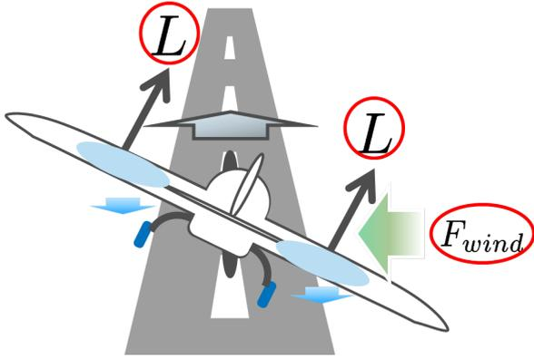
Fig. 2. Overview of sideslip landing
