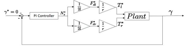
Fig. 8. Block diagram of yaw feedback controller
