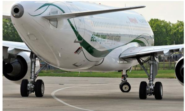
Fig. 1. Electrically driven wheel of Airbus A320<sup>(2)</sup>
