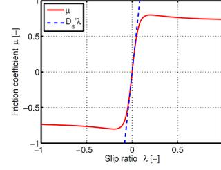
Fig. 2.  $\mu$ - $\lambda$  Curve.
