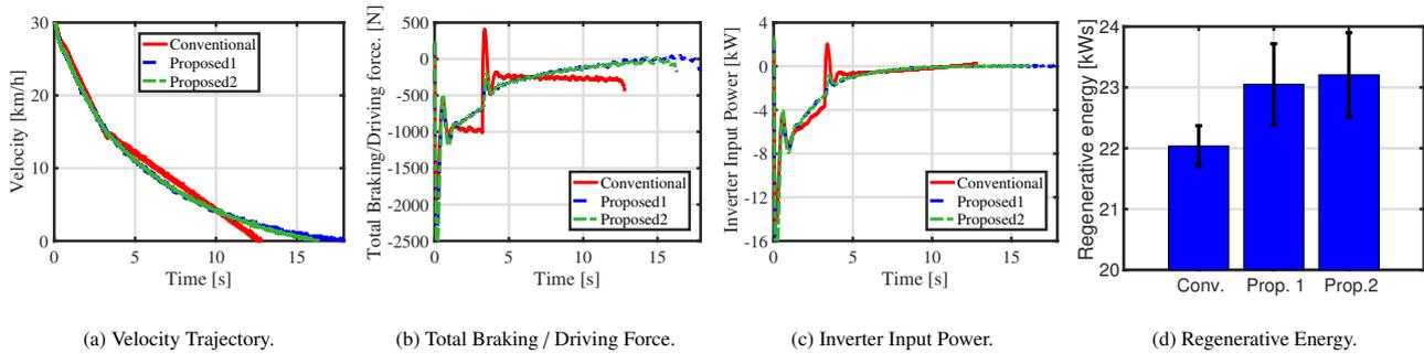
Fig. 7. Experimental Results of RC-S.
