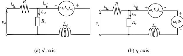
Fig. 3. Equivalent Circuit of PMSM.
