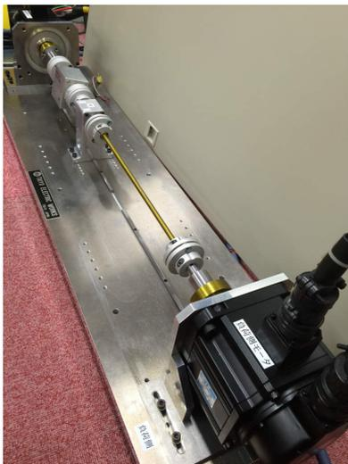
Fig. 4. Experimental setup of two-inertia system
