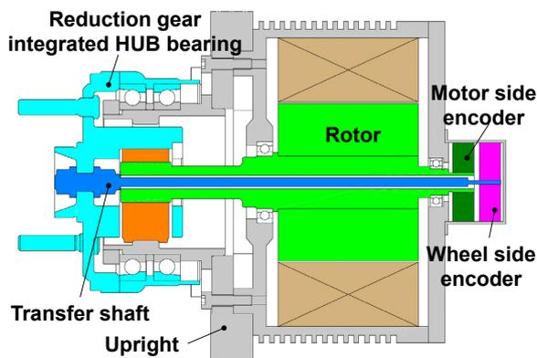
Fig. 6. In-wheel motor unit with load-side encoder
