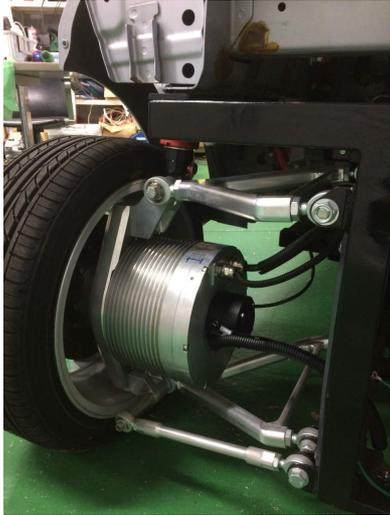
Fig. 5. In-wheel motor electric vehicle with load-side encoders
