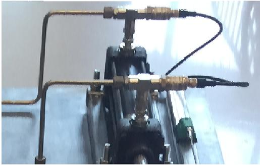
Fig. 3. Experimental setup of valve-controlled hydraulic cylinder with pressure and displacement measurement
