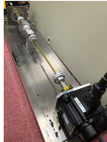
Fig. 1. Outlook of a two-inertia system motor bench.
