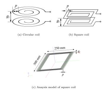
Fig. 4 Double layered open end spiral coil
