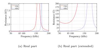
Fig. 9 Impedance frequency plots of 85 kHz self-resonant open end coil (Real part)
