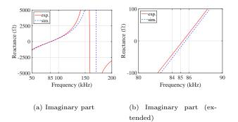
Fig. 8 Impedance frequency plots of 85 kHz self-resonant open end coil (Imaginary part)
