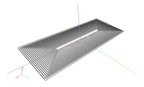
Fig. 10 Analysis model of short end coil on IE3D
