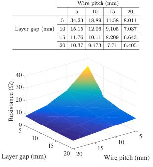
Table 5 Simulated AC resistance at 85 kHz
